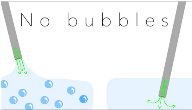
Fig. 6 Injecting the material while keeping the tip inside the material we just extruded, significantly reduces the chances of creating bubbles inside the material.
